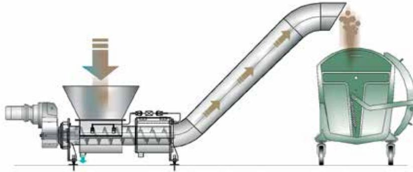
Screenings fall into the compactor hopper from which a rotating shafted spiral conveys solids to the compacting zone where they are dewatered and, at the same time, conveyed to the outlet. The compacting zone is equipped with spray nozzles for washing organic matter contained in the screenings. The liquid produced by washing and compacting is transferred back to the purification process through the screening channel.
